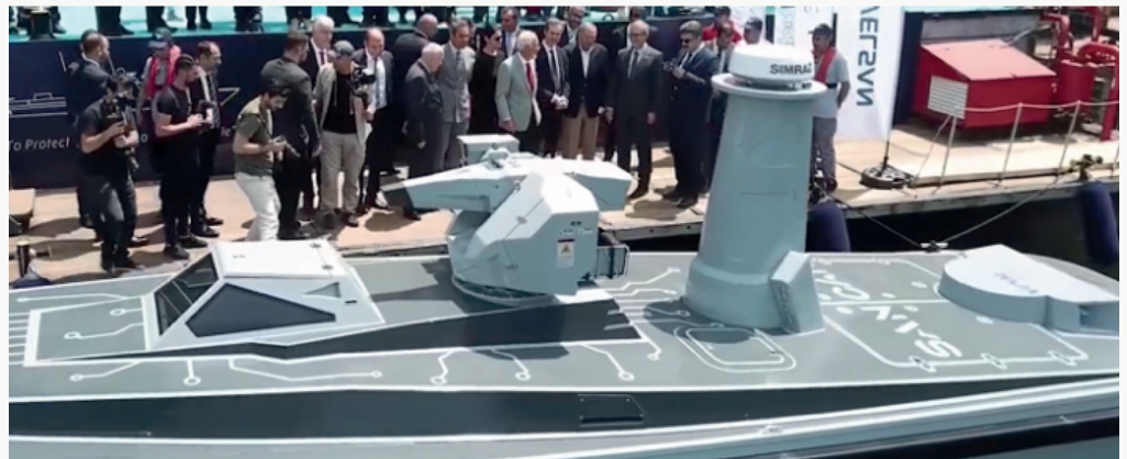
SANCAR USV's Weapon Configuration (including ASELSAN STAMP-2 and MILMAST Telescopic Prop 34 )
